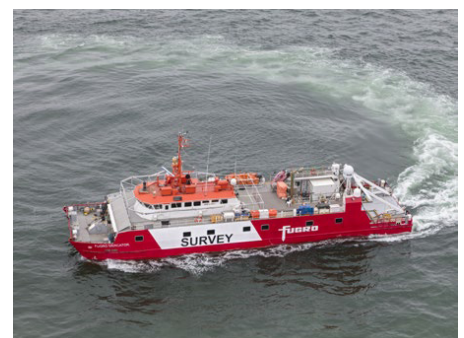
The Fugro Mercator is a custom-built 42 m survey vessel
