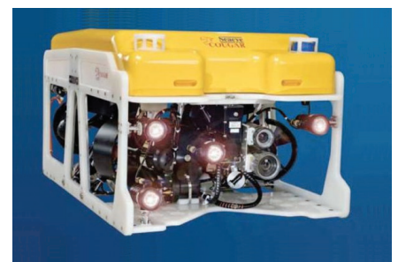
The rugged polypropylene and stainless steel chassis is maintenance free.
