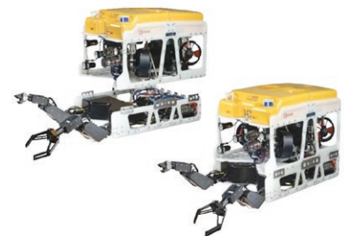
Quick change underslung skirts allow the Cougar XT to perform a variety of light tooling or survey works.
