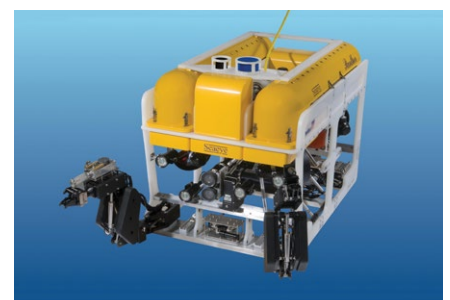
The 2 electronics pods provide most of the Panther XT buoyancy. Additional buoyancy is provided by shaped syntactic foam blocks.
