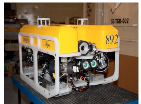
Compact and highly maneuverable, the Seaeeye Tiger is an ideal tool for Visual inspection tasks.
