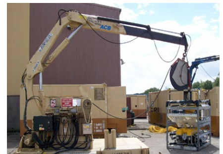
Gravity based deployment systems suitable for operations in Seastate 6.
