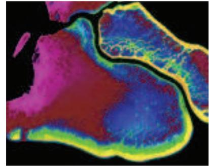
**Above: Satellite-derived bathymetry of Great Barrier Reef from reef crest down to approximately 25m water depth. Below: Sea-floor reflectance of Great Barrier Reef**
