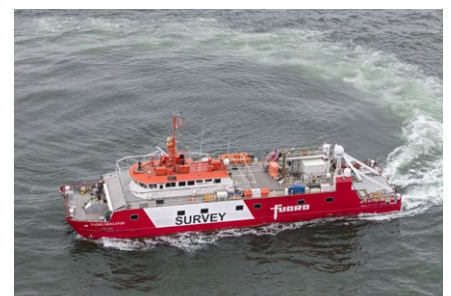
The Fugro Mercator is a custom built 42m survey vessel.
